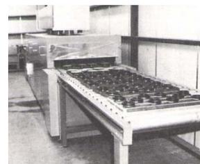
Drying of automobile rear mirror & side mirror paint coating
